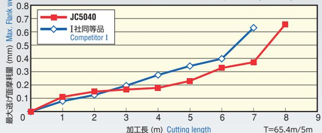
被削材 Material: SKD11 (生材) 1.2379 (raw material),
