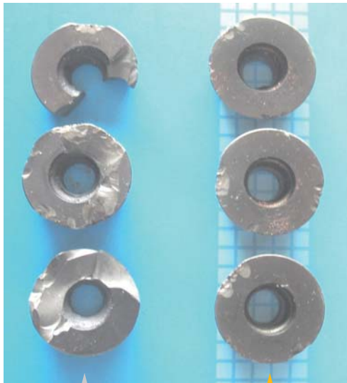
Conventional tool Insert thickness 4.76 mm.
